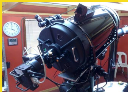
ST10XME with AO8 adaptive optics on C14
