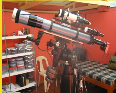
Astrophysics 5 inch f8 Starfire, Borg 77ED f4.3, Titan mount, STV autoguider, Atik 16HR camera
