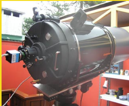
DBK21 webcam on C-14 for high resolution planet imaging
