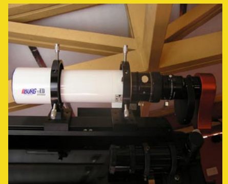
Borg 77ED f4.3 with helical focuser and ATK16HR
